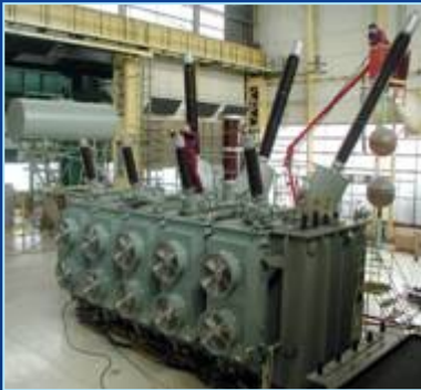
SS ERNESTINOVO AUTOTRANSFORMATOR 420 kV/ 300 MVA CROATIA
