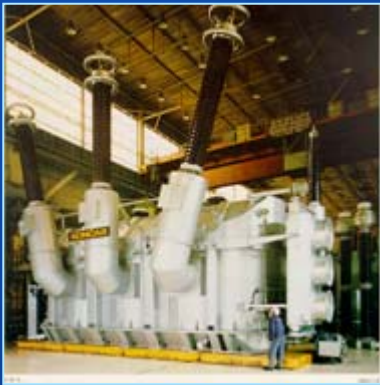
TPP OBRENOVAC 420 kV/ 725 MVA SCG
